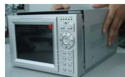
2. Remove the unit cover.
