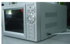
1. Loosen the screws.
